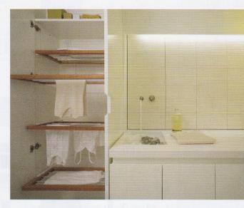
The focal point of the sleek, white space is a glowing laundry chute (left) illuminated from within by fiber-optic cables. The Pyrex tube was produced by a manufacturer of laboratory vacuum equipment and was sand-blasted from the inside to contain the
